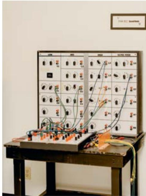
Left: An antique passive crossover cart, once used by loudspeaker engineers to design crossover networks (which split audio into two strands), stands in a corridor at Harman's Northridge facility
