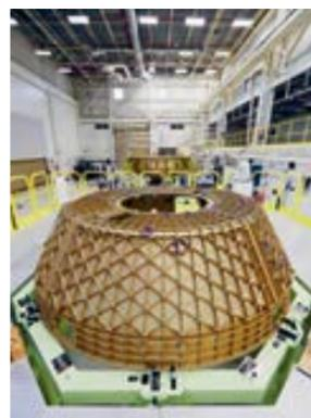
Above: An image of the CST-100 is displayed onto a hangar wall at the opening of the C3PF. Left: A section of the Boeing CST-100 Structural Test Article rests on a test stand
