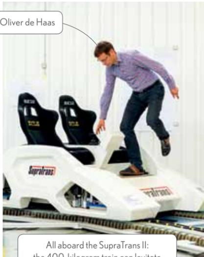
All aboard the SupraTrans II: the 400-kilogram train can levitate about 10 millimeters above its oval track.
