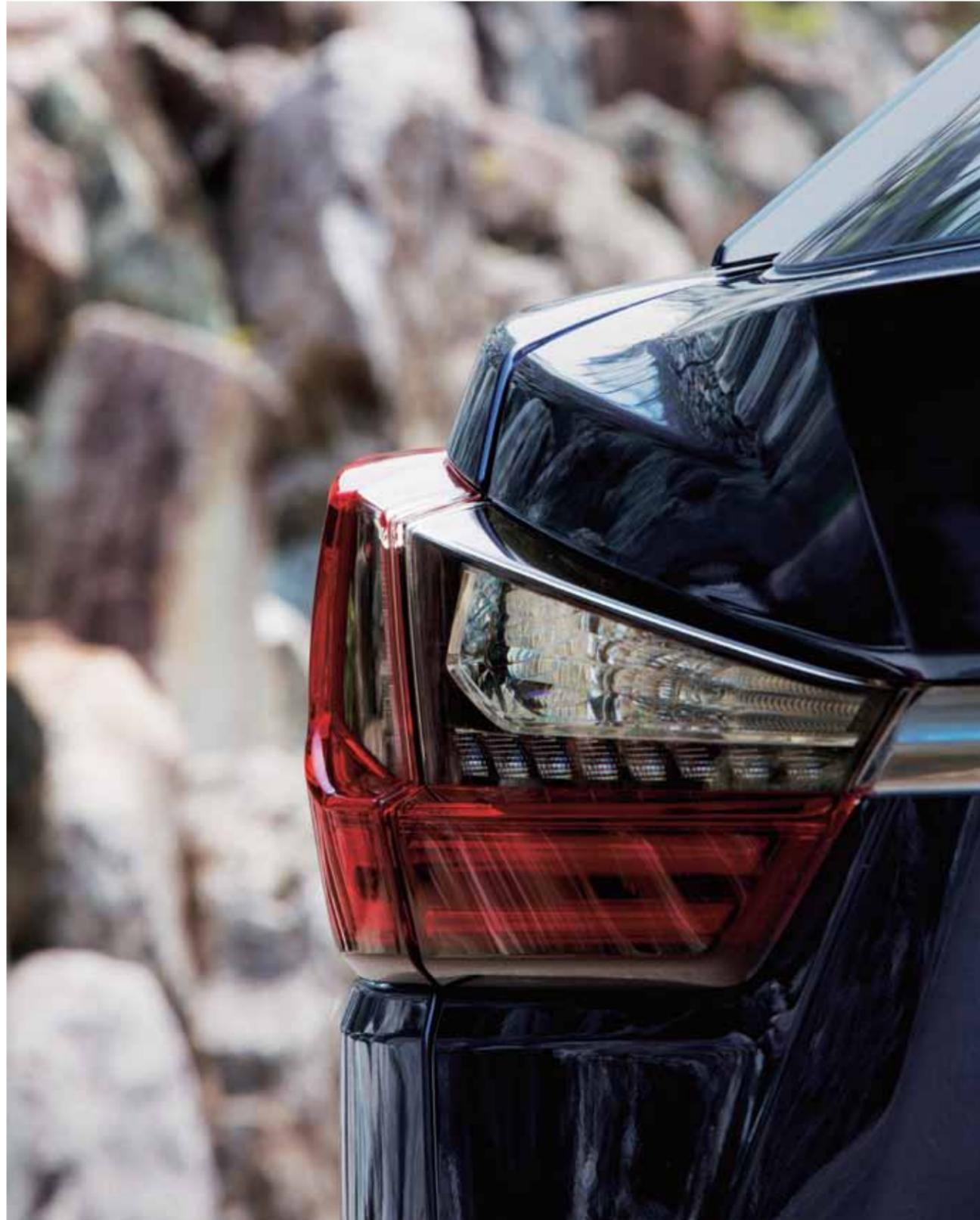
Meticulously crafted, the jewel-like taillights of the high-grade RX highlight a totally restyled end. The LED turn signal lights are sequential: meaning they illuminate in order from the inside to the outside, conveying the change in direction of travel.
