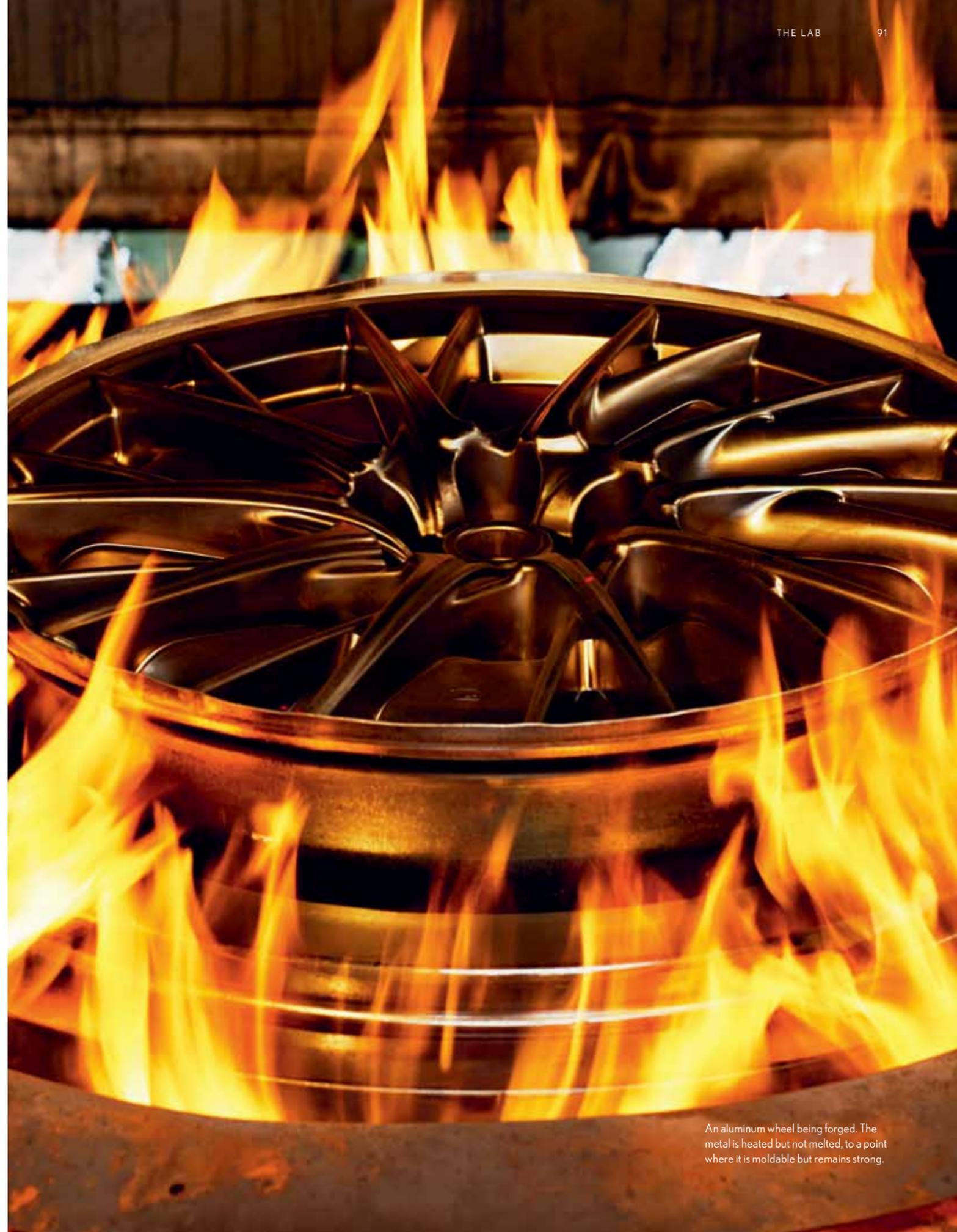
An aluminum wheel being forged. The metal is heated but not melted, to a point where it is moldable but remains strong.
