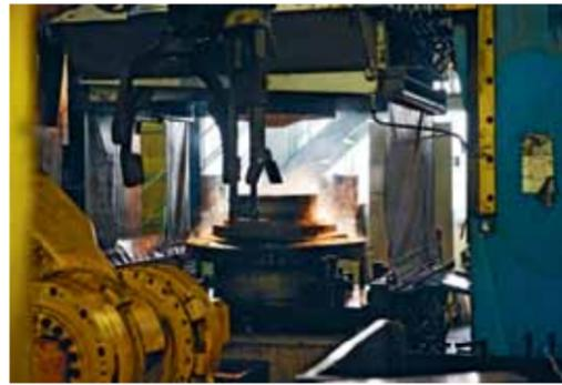
Above and right: Wheels being made at the Takaoka factory are shown at different stages of the forging process.
